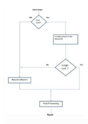
FIGURE 03 Arabic Text Recognition flow
